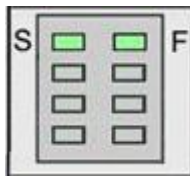
Figure 8: Power Module LED Indicators
