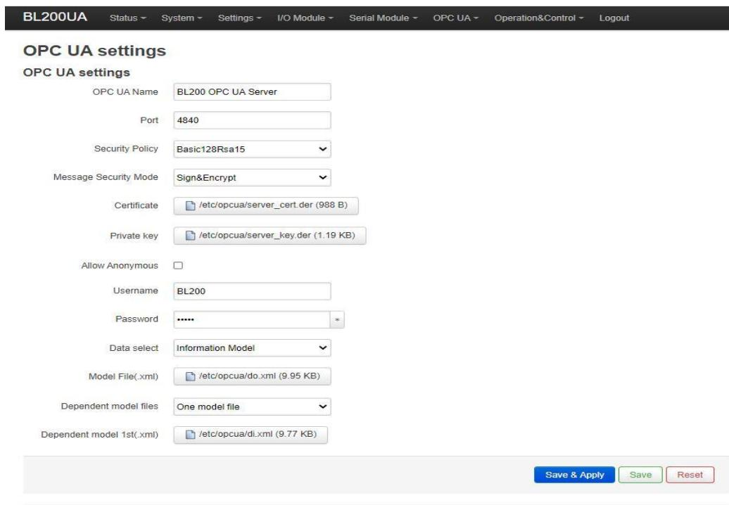
The screenshot shows the 'OPC UA settings' configuration page for the EdgeIO BL200 Series. The top navigation bar includes links for BL200UA, Status, System, Settings, I/O Module, Serial Module, OPC UA, Operation&Control, and Logout.
