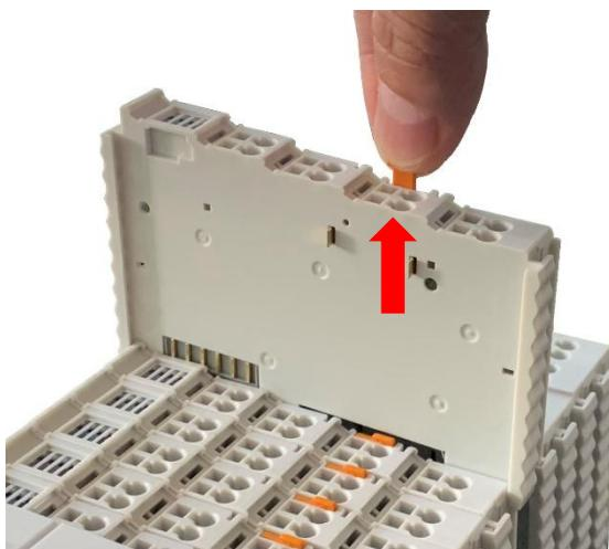
When the I/O module is removed, the electrical connection to the data or power jumper contacts is disconnection.
