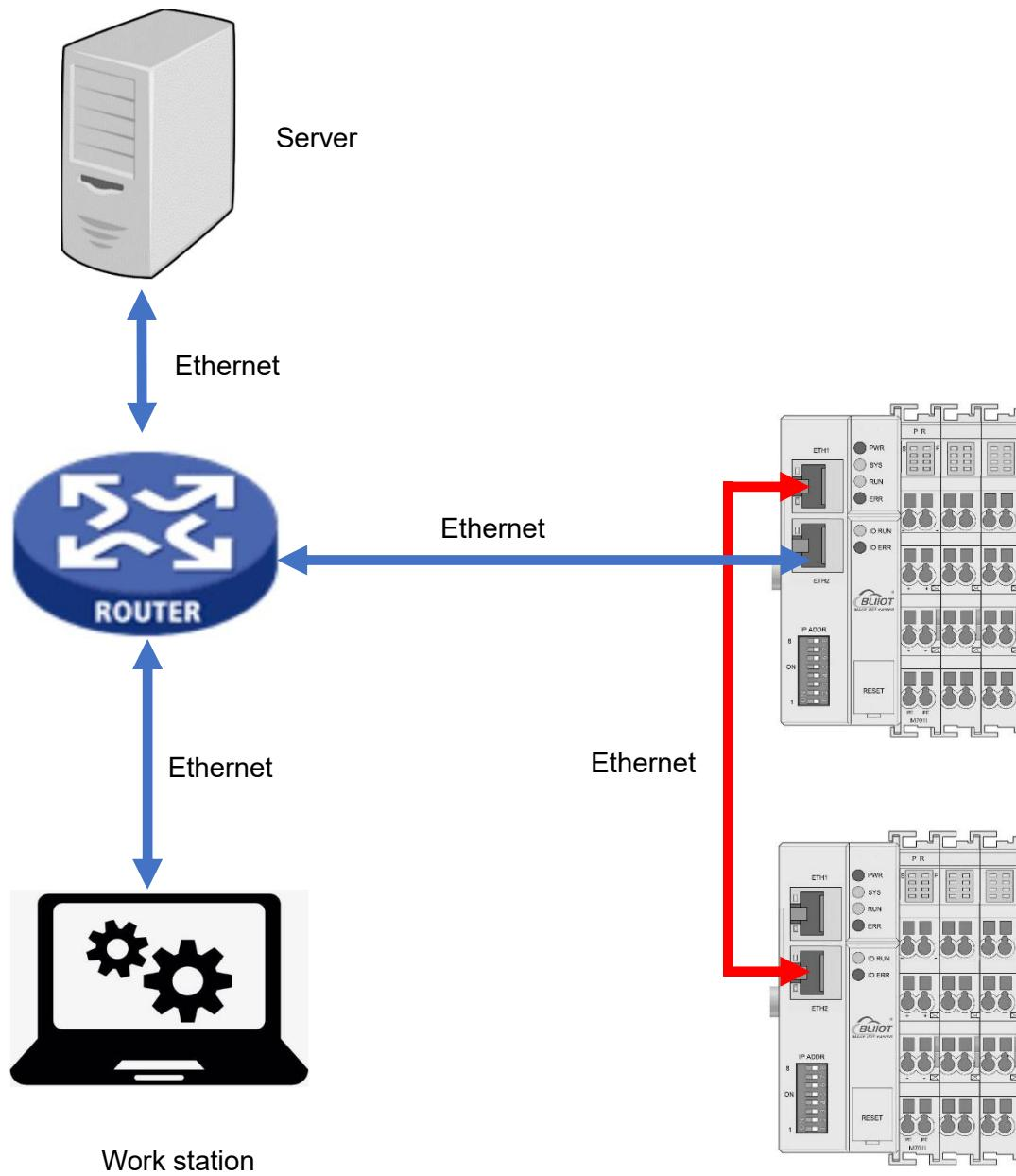
Directly connected to the computer through ETH 2.
