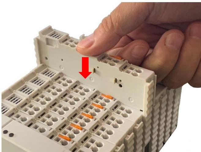
After the I/O module is installed, the electrical connection to the coupler (or the previous I/O module) and the following I/O module is established via the data contacts and the power jumper contacts.
