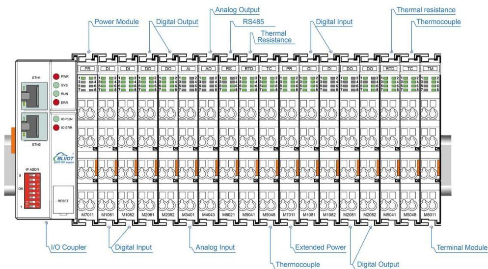
The communication between the node and the field devices (eg PLC) takes place via the Ethernet interface of the fieldbus coupler, and the communication between the fieldbus coupler and the I/O modules takes place via the local bus. The two Ethernet interfaces are internally integrated with a switch function, which can establish a linear topology without the need for additional switches or hubs.
