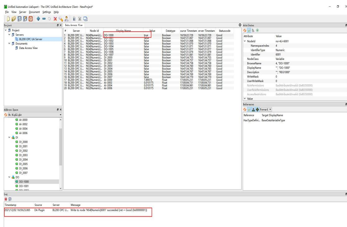
Check the DO status in the web configuration of BL200. DO1 is also changed from the original open to close.
